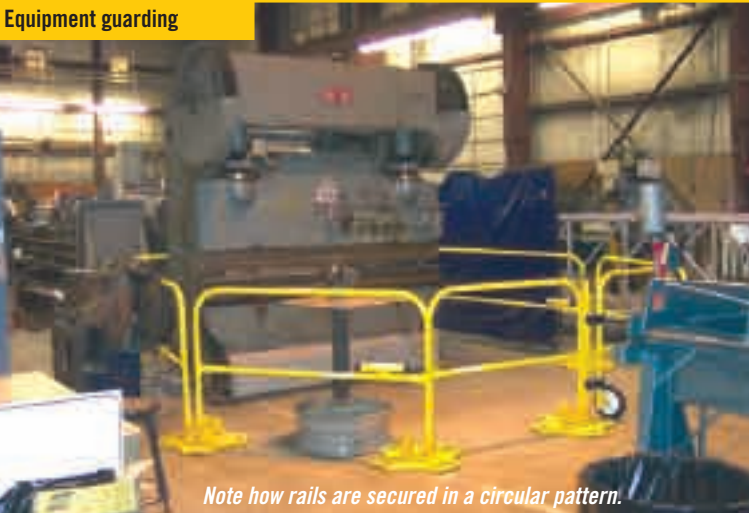
Note how rails are secured in a circular pattern.
