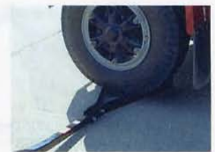
The wheel pad anchored with a service vehicle's weight,
